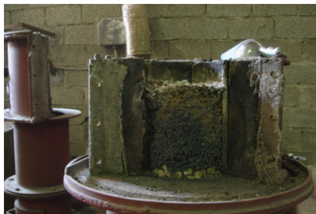
Fig. 5. View of the opened sinterpot with the formed sinter cake inside.
