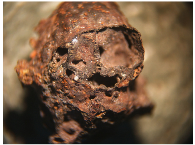
Fig. 8. Glassy phase formation on the outer surface of sintered pellet.
